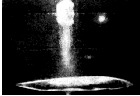
Figure 5. Change of the EGB wave diameter under avalanche-streamer transition [7].
